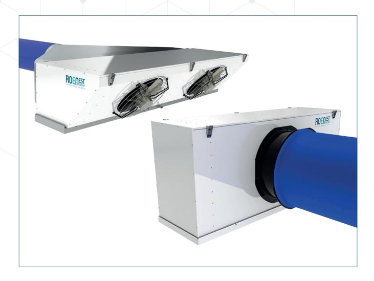
These air treatment and distribution systems consist of special air cooling units combined with fabric diffusion ducts. The assembly is designed to provide the required thermal power and air flow rate, achieving optimal diffusion while minimising noise and power consumption. The air cooler is made with a double insulated tray, pre-painted aluminium casing, stainless steel metalwork and diffusers with anti-condensation treatment.
